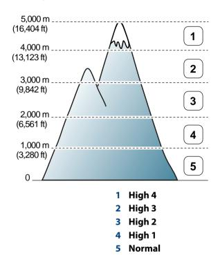
You can set the altitude value from **Device Settings** in Samsung Easy Printer Manager program or **Machine** section in Printer Settings Utility program.
